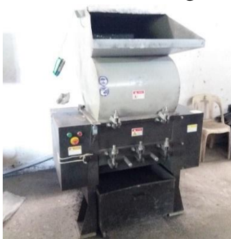
Plastmassa maydalagich 1-ikkilamchi xom ashyo, 2- maydalagich tishi, 2- kechuvchi tig', 4-rotor vali, 5 –korpus.
