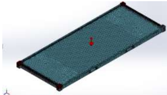
Figure 2 . Container-platform body structure finite element model
