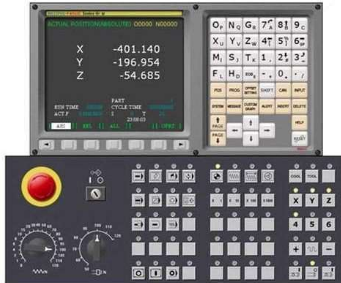
Figure 3. Writing a control program using the CNC drilling machine and its control panel.
