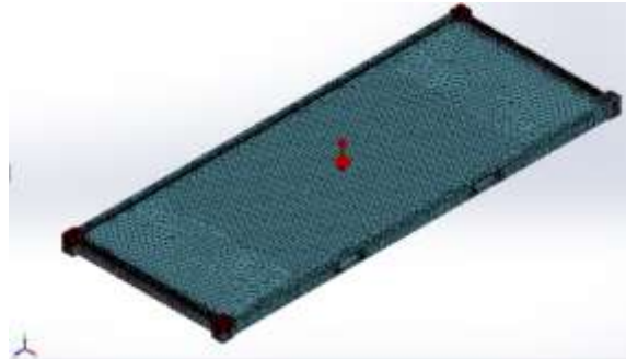
Figure 2 . Container-platform body structure finite element model
