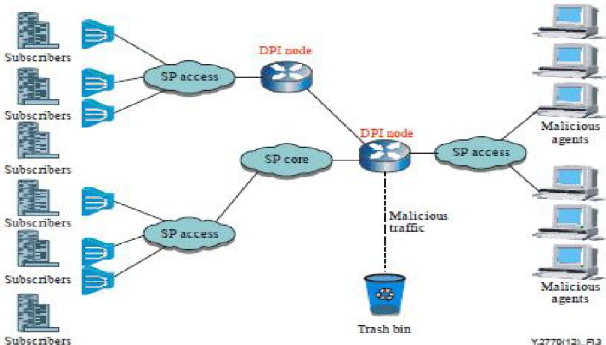
**1-rasm. DPI qurilmalarining ishlash prinsipi.**
