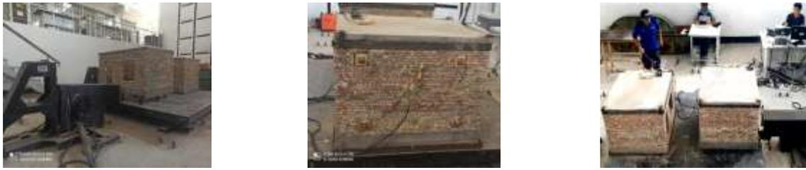
**Figure 3.** Built-in models of buildings (a), the state of installation of measuring sensors at characteristic points (b) and the process of excitation of small vibrations (c)
